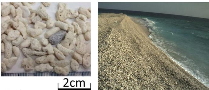
Fig. 1 Coral gravels at laboratory scale (Tajima and Fujikawa, 2016), left; and Coral gravel beach at Ballast Island (Fujikawa et al, 2015), right.
